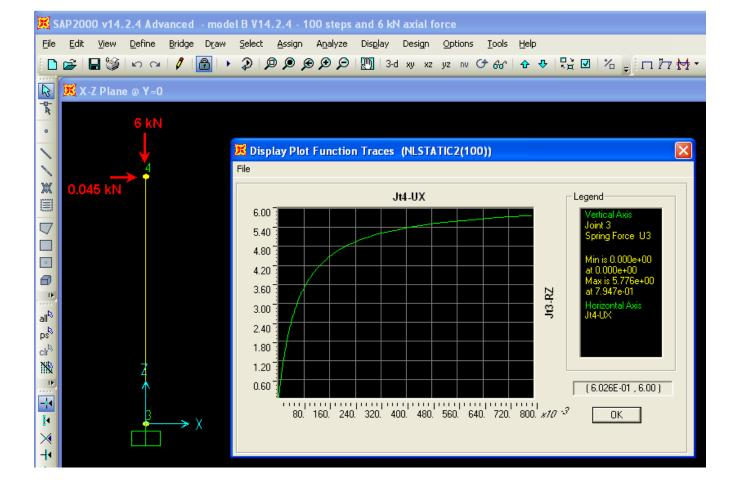
Users may download the analytical model for this system through the P-Delta effect for fixed cantilever column test problem.
