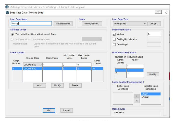
Figure 1: Moving load case definition
