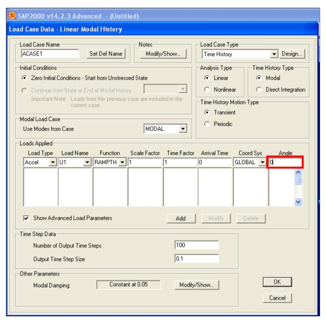
Figure 1 - Angle specification for time-history acceleration load
