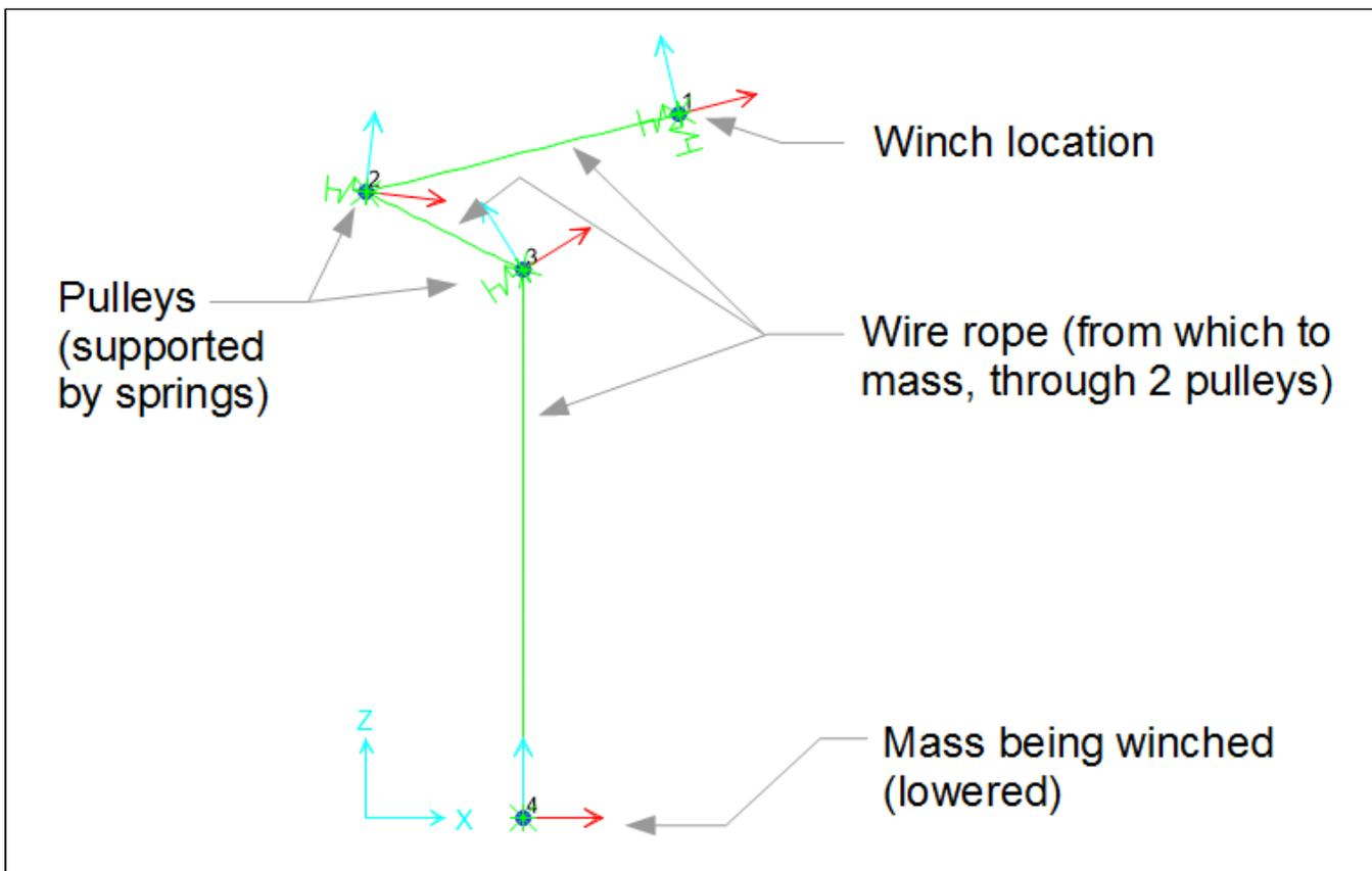
Figure 1: Geometry of the pulley assembly
