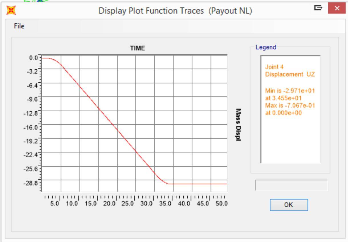
Figure 2: Mass displacement
