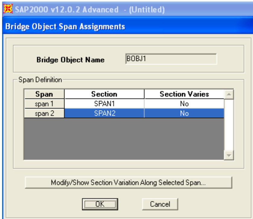
Figure 3 - Span assignments
