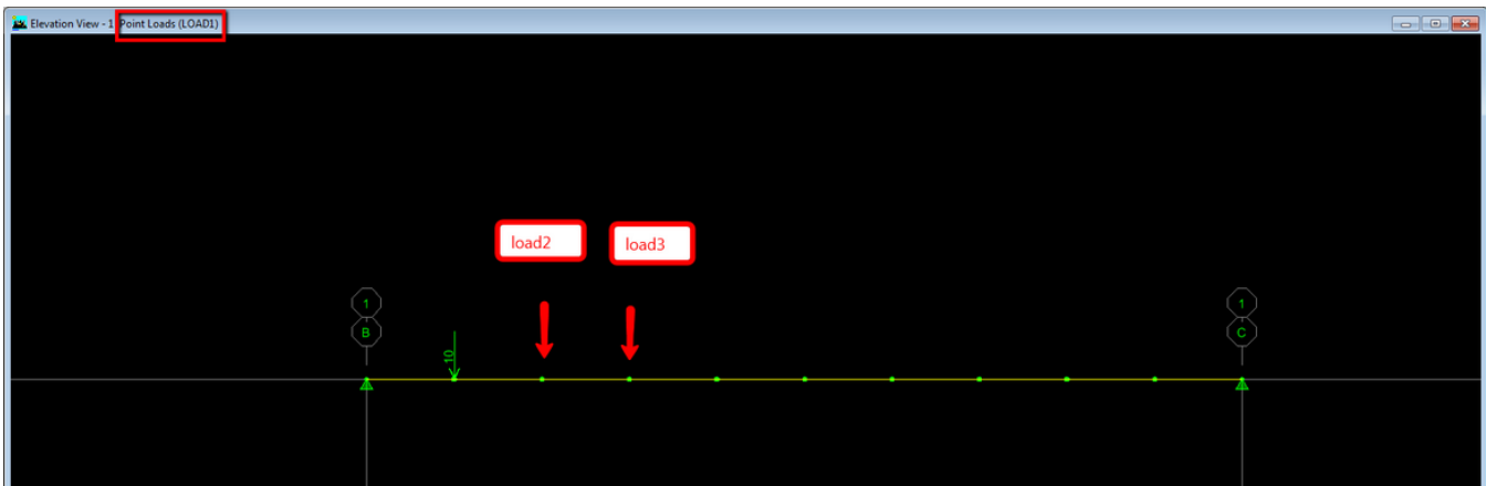
Figure 1 - Modeling the moving load
