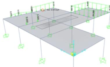
with load-size assignment may be superimposed on punching shear locations. At the foundation level, checks are run for punching shear from piers and piles. Nonlinear uplift can be implemented through soil-spring modeling. Manual and automatic point, line, and uniform loads, enveloped and applied per user-defined or building-code specification, are presented in clear and detailed 3D views.
