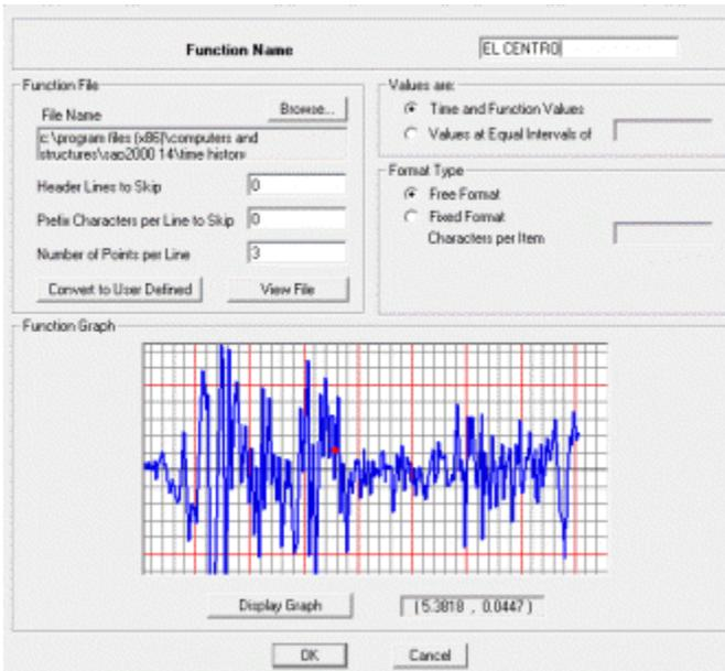
features for nonlinear and dynamic consideration. This versatility makes SAP2000 a practical and productive tool for any analysis type ranging from simple static, linear-elastic to more complex dynamic, nonlinear-inelastic.
