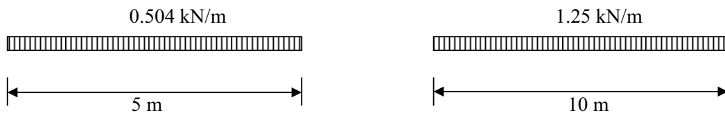
Line Loads for Live Load Q (left) for Purlin, (right) for Rafter
