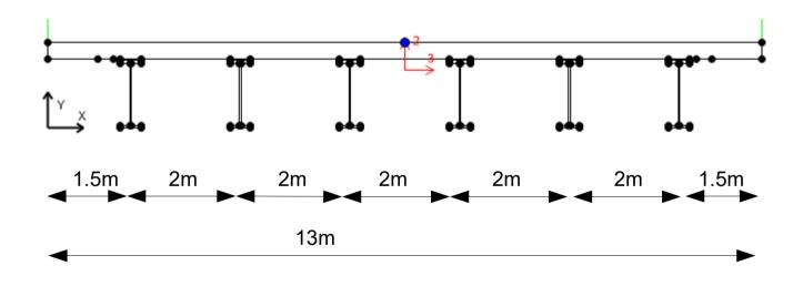
Base Deck Dimensions (Before Applying the Parametric Variation)
